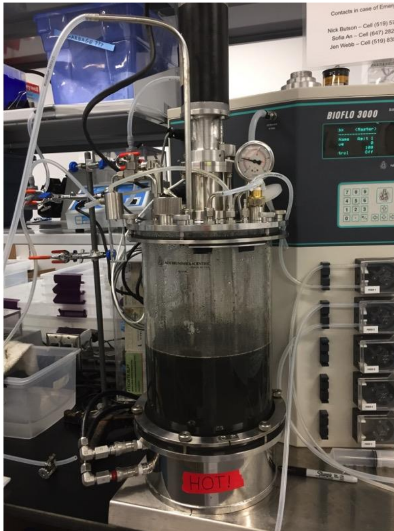
Figure 2-1: The lab scale anaerobic digester owned and operated by Geosyntec Consultants is displayed in this photo.
