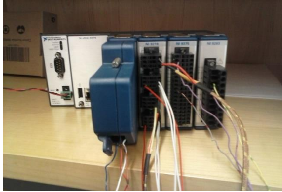
Figure 65: Lab-Scale PAMS Set-Up with NI Equipment
