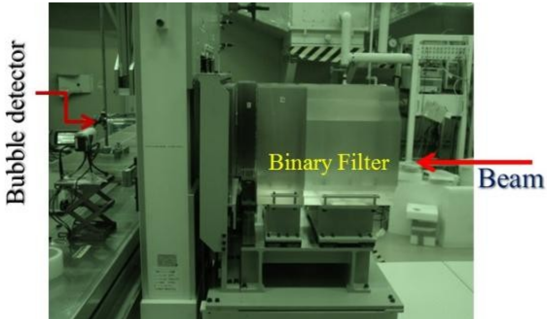
Figure 25: Experimental setup with space bubble detector at HIMAC
