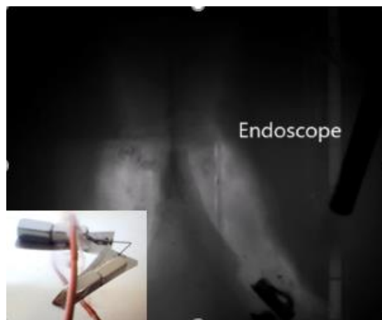
Figure 44: The brain tissue of a goat is clamped inside the agar mold while the pair of scissors is used to cut the protruding tissue. The inset shows the image taken from the endoscope.
