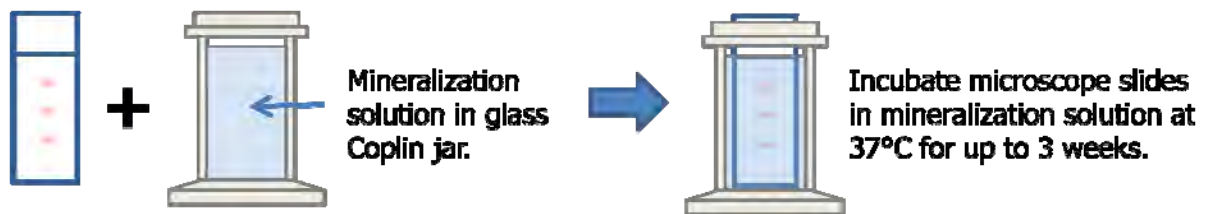
Figure 6 Experimental set-up for re-mineralization and 2 nd de-mineralization.
