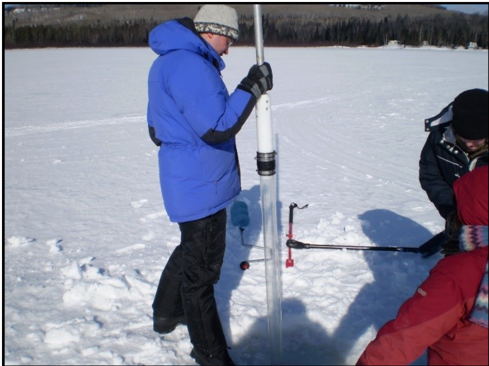
Figure 5.5 Universal corer used to extract the short core.
