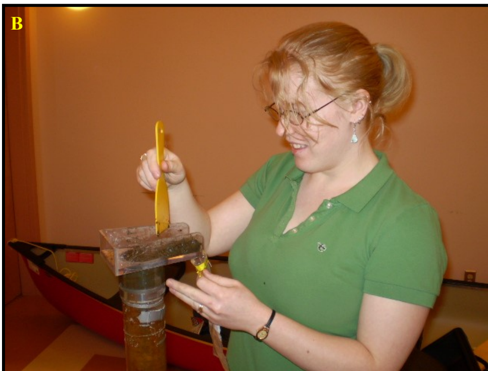
Figure 5.6 Sampling the short core, WTFSH08-02, to be sub-sampled later for pollen and phytoliths processing in the lab.
