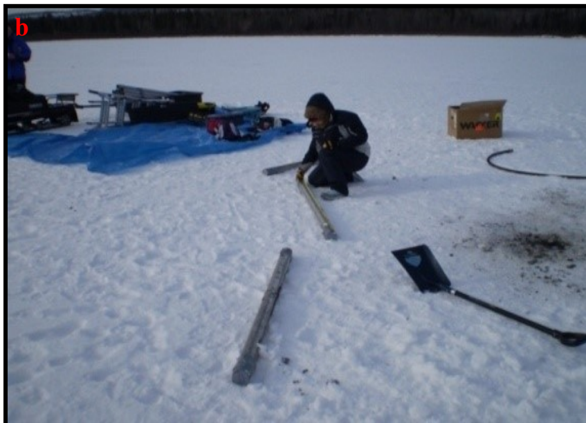
Figure 5.3 Preparing core WTFSH08-01 for storage: photo A) cutting the long core into manageable sections; photo B) measuring and labelling core sections
