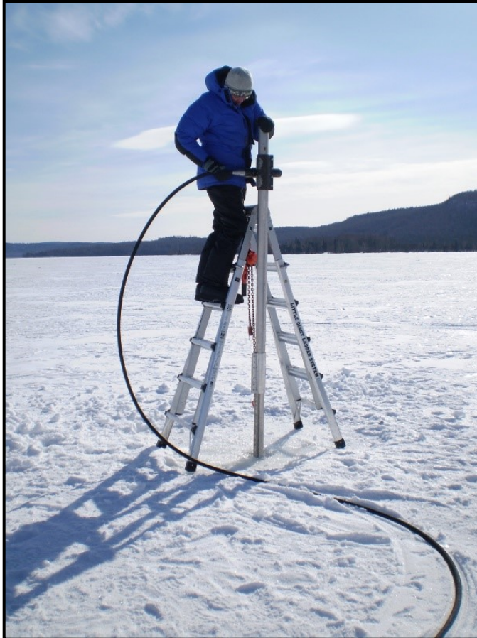
Figure 5.2 Assembling the core and adding sections of aluminum pipe.
