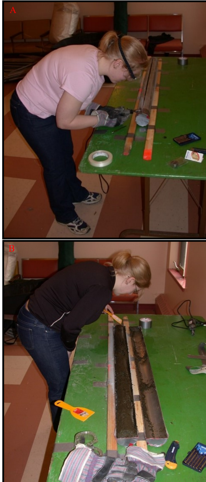
Figure 5.4 Photo A) Splitting the core barrel, photo B) examining the sediments.
