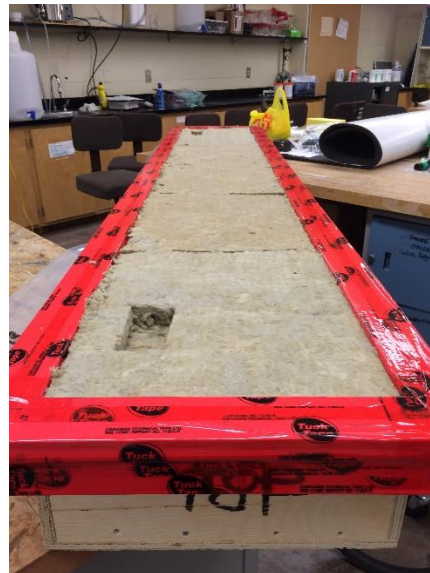
Photograph 2: View of test box loaded with mineral fibre insulation.
