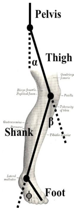
**Figure 2: The definitions of joint angles used by Hawkins and Hull [1]. The hip angle ( $\alpha$ ) is between the pelvis and thigh, the knee angle ( $\beta$ ) is between the thigh and shank, and the ankle angle ( $\phi$ ) is between the shank and foot. The dotted lines represent the imaginary extensions of the limb segments. The original anatomical image was taken from the work of Gray [2].**
