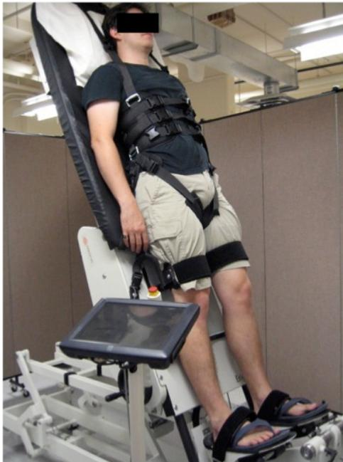
**Figure 15: A harnessed participant under 70-degree head-up tilt.**
