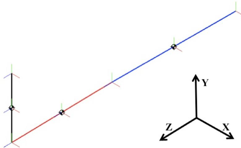
**Figure 3: The isometric view of the geometrical representation of a lower extremity in a commercial simulation environment. The links representing the foot, shank, and thigh are colored as black, red, and blue, respectively. The y-axis of the inertial reference frame points against the direction of the gravitation acceleration, and the z-axis points along the long bones of the leg and toward the ankle.**
