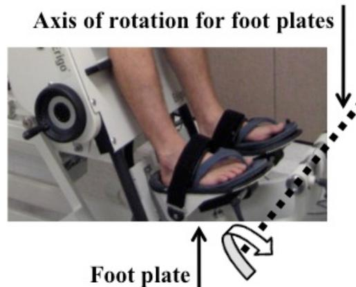
**Figure 14: Foot plates and their axis of rotation.**
