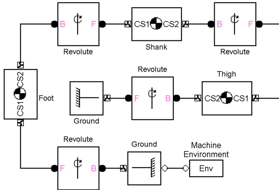
**Figure 4: The block diagram of a lower extremity, as implemented in a commercial simulation environment. Each revolute joint represents a rotational degree of freedom in the sagittal plane. The toe of the foot link and the proximal end of the thigh link were connected to the inertial reference (ground) via a revolute joint.**
