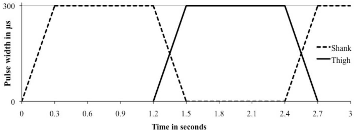
**Figure 1: The stimulation pattern for the isometric FES intervention. The two complete waveforms comprise one cycle of stimulation. The cycle was repeated for the entire duration of the isometric FES intervention. The dashed line represents the stimulation of the tibialis anterior and calf muscles, and the solid line represents the stimulation of the quadriceps and hamstring muscles. The stimulation was symmetrical between the two legs.**
