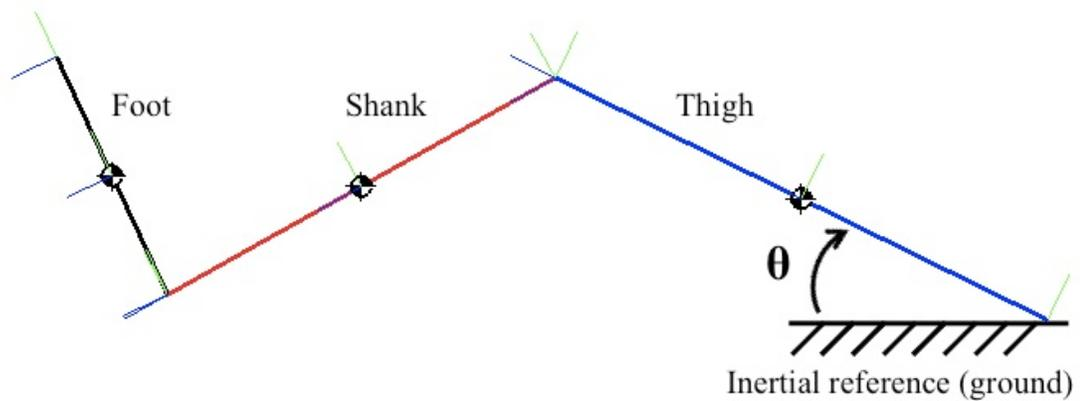
**Figure 6: The linked-segment model of the leg, as implemented in a commercial simulation environment. The thigh angle (labeled as  $\theta$ ) was defined as the angle from the horizontal to the thigh link.**
