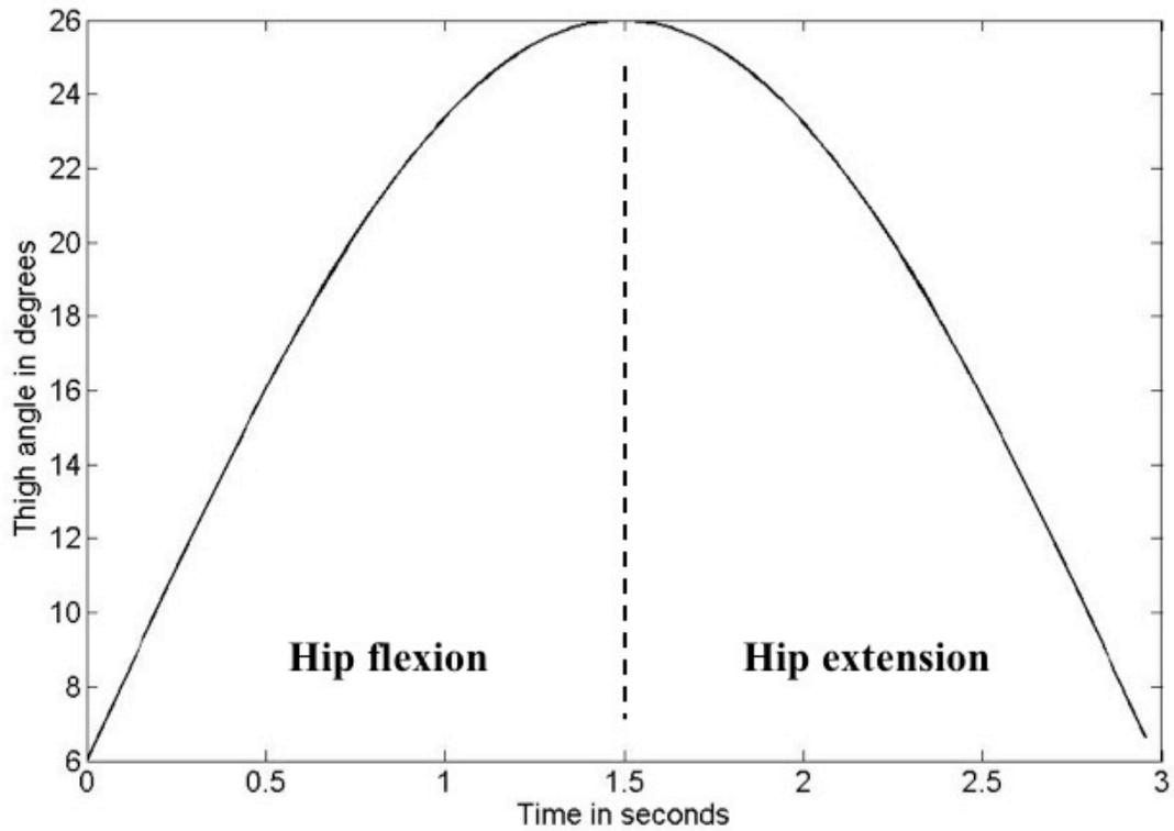
**Figure 5: Sinusoidal input for the thigh angle. The same range (6 to 26 degrees) and speed (40 steps per minute) of motion as those used in the experimental protocol.**
