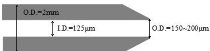
Figure 3.2.3 Geometry of ESI emitter.
