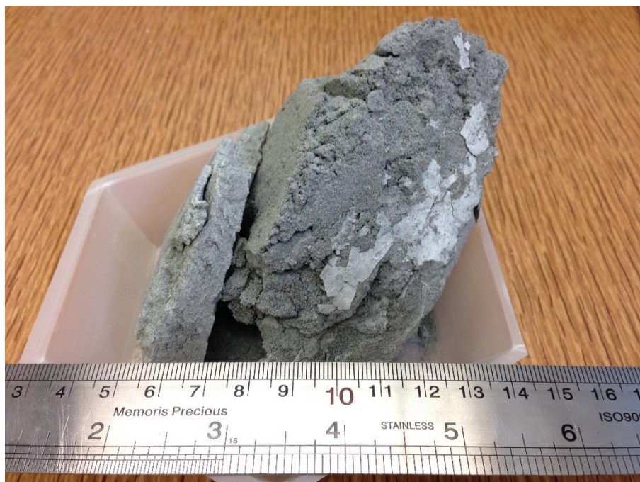
Figure S2. Photograph of spent NiMT progressively accumulated over 2 years from the diffusive batch cell and representing ca. 70 room-temperature wet carbonation runs to evaluate the long-term stability of the carbonates. The samples were left open in laboratory conditions.
