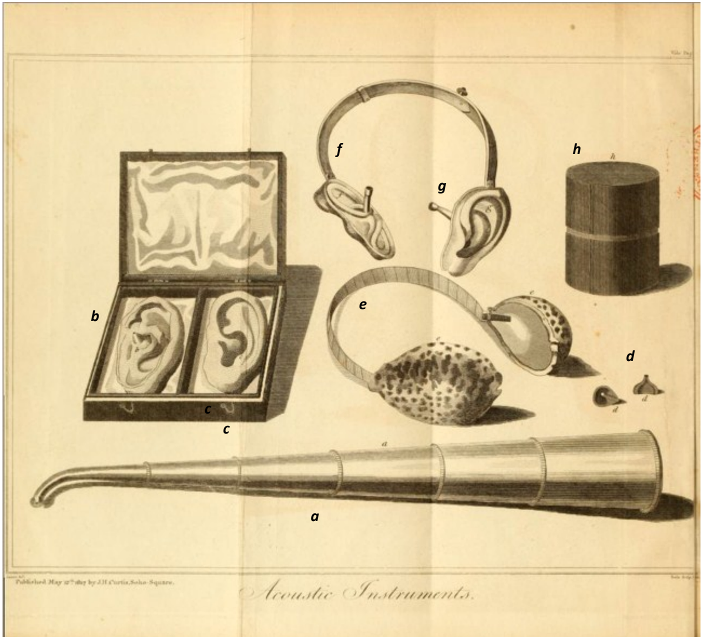
Image 11: Various acoustic instruments devised and/or marketed by John Harrison Curtis. From the frontispiece of his Treatise (1817): (a) Collapsible Hearing Trumpet (b) French artificial ears with gold tube, internal side (c) French artificial ears with gold tube, external side (d) the tubes (e) Spanish ears (f) internal part of German silver ear (g) external part of German silver ear (h) trumpet case.
