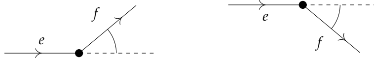
Figure 3.6: A positive turn angle (left) and a negative turn angle (right). If e = -f , the turn angle is +180^\circ by convention.
