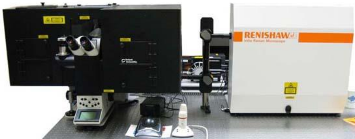
Figure 3.1 The Renishaw inVia Raman system equipped with a Leica microscope (left) and a Renishaw spectrometer (right).
