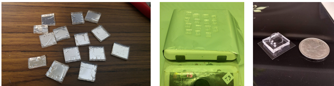
Figure 6.3: Left: Individual poly(dimethylsiloxane) (PDMS) devices cut from a larger disc. Middle: Post-bake following oxygen plasma exposure. Right: A completed microfluidic chip with waveguide inserted. A coin is provided for scale.
