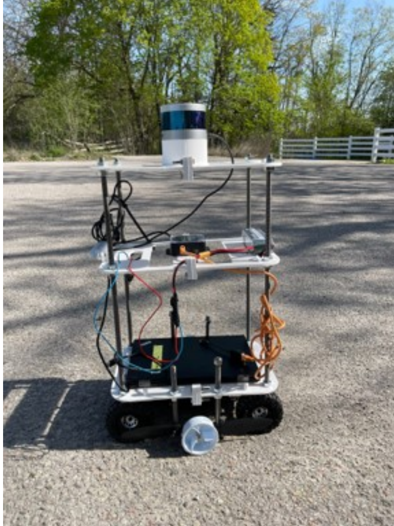
Figure 3.13: Designed mobile platform used for gathering the data in the second dataset.
