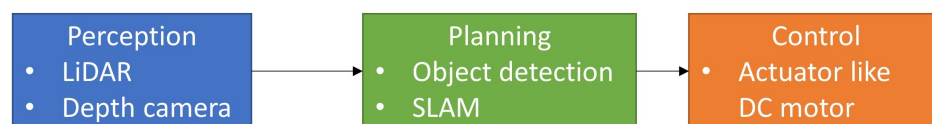
Figure 1.1: This figure shows different components of autonomous systems including perception, planning, and control.
